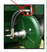
The oil flow control valve is factory set in the fully closed position. It must remain in the fully closed position unless the tractor is fitted with a fixed displacement (open centre) hydraulic system.
