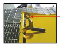
Over centre adjustment is achieved by adjusting the eye of the latches in or out until desired pressure is obtained.
