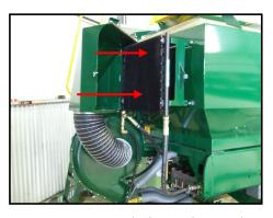
The hydraulic oil cooler fitted to all Simplicity Airseeders should be periodically checked and cleared of trash build up.
