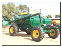
Load/Unload auger in the stowed position
