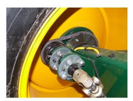
The metering drive system is connected to the drive wheel by an electrically operated mechanical clutch. The clutch requires some maintenance to ensure efficient operation.
