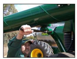
**Step 4**Tighten 'star' nut on rear mount using spanner supplied.
