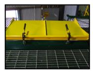
When closing the lids check that the latches close with 'over centre' force. This will ensure that the lids are tight and pressure is applied to the seal.
