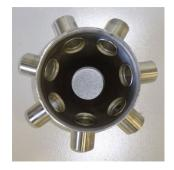
The Secondary Head is manufactured from stainless steel and has either a 44.5mm, 50mm or 63mm internal diameter inlet depending on the uptube and can have 4 to 10 outlets per head. The outlets are 32.5 mm outside diameter to accommodate the terminal lines. The Secondary Head is sealed at the top by a durable rubber cap to avoid seed damage.
