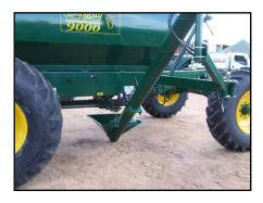
To place auger in an unload position, manoeuvre the auger and the arms so that the hopper can be placed under a bin clean out door.
