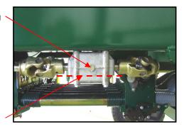
The oil level in each 'T' Box should be checked at the start of the sowing season.
