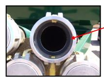
Finally, before reconnecting the primary hoses, make sure that there is a sealing ring in the female section of the camlock as shown.
