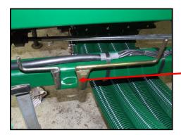
After use stow the calibration crank handle and the compaction crank handle in the position provided at the front of the Air Seeder
