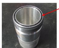
Fit the new head to bowl O ring seal (supplied) to the bowl in the position shown.
