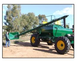
**Step 1**Lift the auger hopper and rotate 90° as shown. Any product left in the auger can be emptied into a container at this time.
