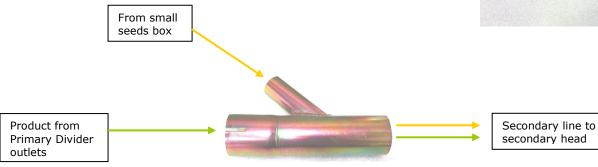
Small seeds induction tubes are a convenient way to place small seed from the small seeds box (option) into the main air streams with the primary product being applied. The blended products then travel via the secondary lines and heads to the sowing boot to be placed in the ground together.
