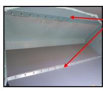
The bin dividers must be fully sealed with silicon as air leaks internally between the bins can be detrimental to the accuracy of the sowing operation. Refer Page 5.1
